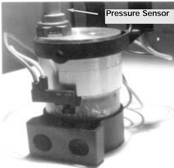
Brake Pressure Sensor Location Bosch DSC III 5.3 (740i/iL, 540i)
